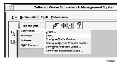
Figure 739-1. Cellworx Vision Connection Menu Tree
